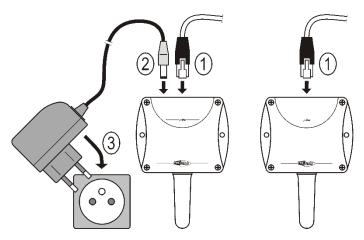
Web Sensor EPND-4S-POE and EPND-3T-POE connection (power supply adapter, Power over Ethernet):
